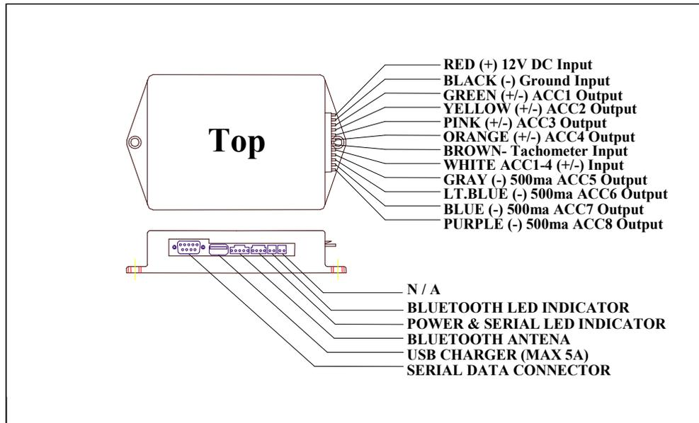
Figure 5: MFC CONNECTOR DIAGRAM
