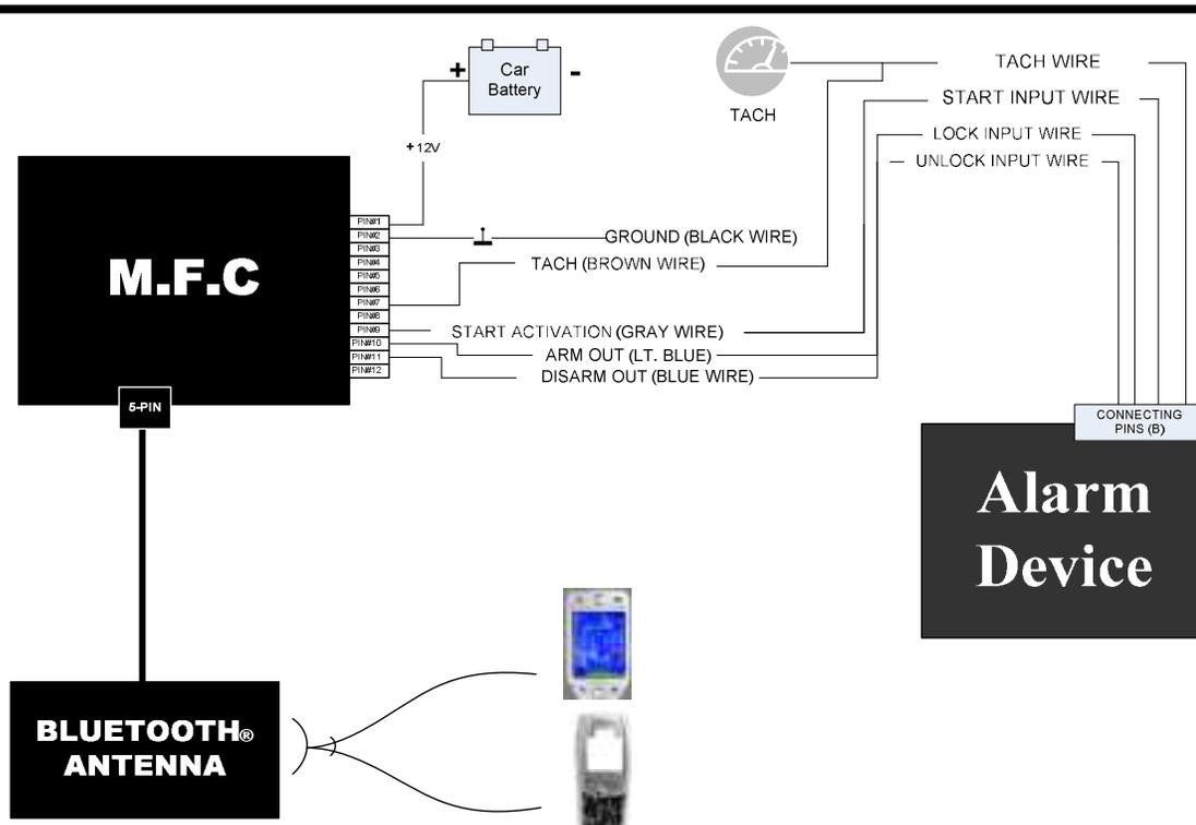
Figure 8: Direct MFC Example: Setup with Alarm add-on
